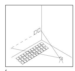
Remove the backing strip from the sticker. Place the Mosaic diagonally against the wall so that it can be positioned at two points equal to the horizontal line. Now press the Mosaic firmly and do exactly the same
