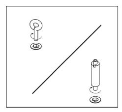
**1.** Screw the screw eyes or connectors into the ceiling island.
