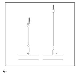
Hang the rigid hangers in the screw eyes OR Push the wire rope through the connector and pull it to the desired distance. By pressing the springloaded part, the wire rope can be pulled back.
