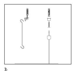
Drill holes in the ceiling at the marked positions and insert the dowels. Screw on the D-rings and hang the rigid hangers from this OR Screw on the upper part of the ceiling mount and twist the lower part onto this with the steel cable pulled through.
